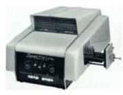
Xenon lamp, variable slits on energisation and emission monochromators, variable scan speeds and recorder... 40 years later, the new SAFAS spectrofluorometers are again introducing new standards in fluorescence.
