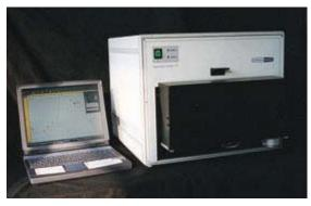
1997 SAFAS® new high peformance flx SPECTROFLUOROMETER, with 2 high speed scanning monochromators, variable slits, high speed 10-cells linear automatic holder, stirring on all the cuvettes, continuously variable slits on both monochromators, instrumental correction and unparallelled sensitivity...
