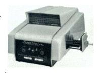
**1968** The world's first automated dissolution testing spectrophotometer for pharmaceutical use was introduced, with automatic 10 cells holder, 8 flow cells, 8-channel peristaltic pump, 8-way recorder, and programmable cycling times.
