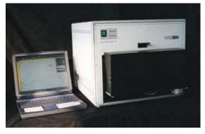
**1997** SAFAS® new high peformance flx SPECTROFLUOROMETER, with 2 high speed scanning monochromators, high speed 10-cells linear automatic holder, stirring on all the cuvettes, continuously variable slits on both monochromators, instrumental correction and unparallelled sensitivity...
